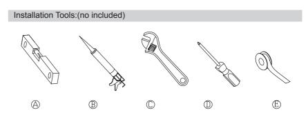
A: Gradient B: Sealant C: Adjustable spanner D: Screwdriver E: PTFE tape
