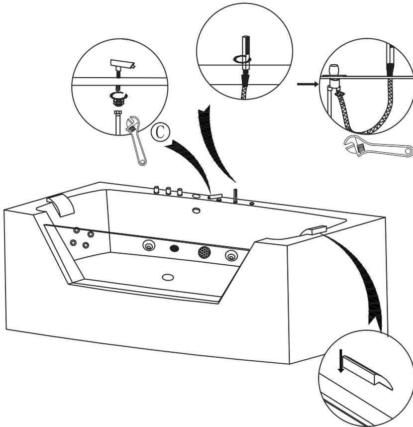
3. Adjust the tub feet to make the horizontal. Move the bathtub to the wall corner; put the drainer into sewer and seal the drainer with sealant. Seal the gap between the bathtub and the wall with sealant to avoid water leakage.
