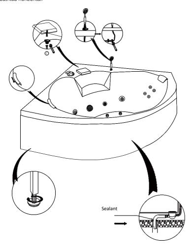
3. Seal the gap between the bathtub and the wall with sealant to avoid water leakage.
