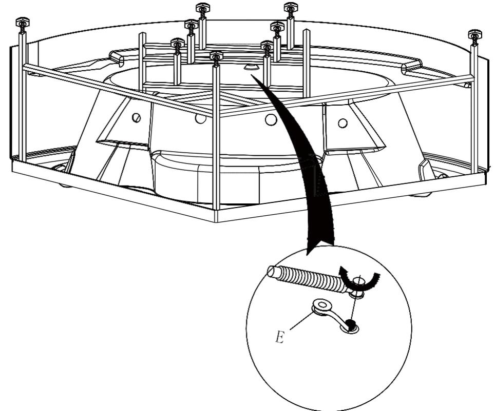
2. As the picture shows below, turn back the bathtub. Install the waterfall, pillow and hand shower, and connect to the water hose. Move the bathtub to the wall corner; put the drainer into sewer and seal the drainer. Adjust the tub feet to make the bathtub horizontal.
