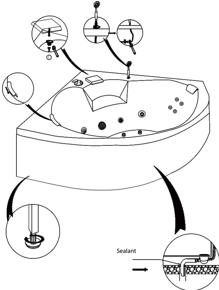
3. Seal the gap between the bathtub and the wall with sealant to avoid water leakage.
