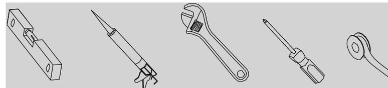
A: Gradient B: Sealant C Adjustable spanner D: Screwdriver E: PTFE tape
