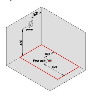
Step 2: Put the bathtub in the corresponding position, leveling with leveling instrument
