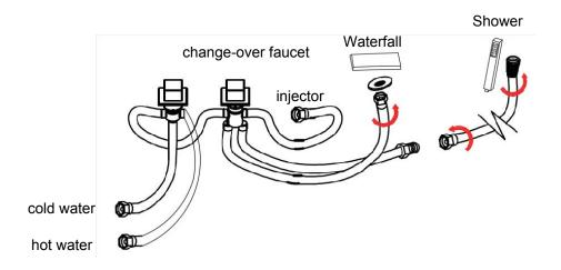
Step 4 : as the pics ,First, Take the down-flow pipe inserted into the sewer ,then connect the inlet pipe (take care the hot and cold water ) and Plug the power cord into
