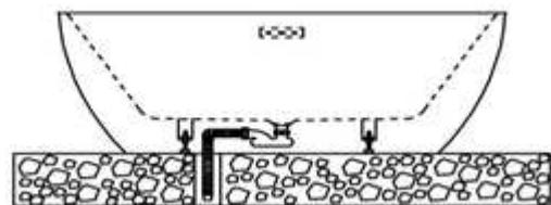
4. After the installation, please test the bathtub by filling it with water. If it drains properly and completely, the bathtub has been installed correctly and is ready to be used.
