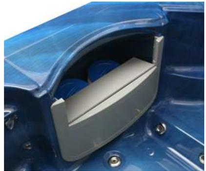
Every 2 months, more often with heavy use, filter must be cleaned to get rid of objects and particles that are lodged in the filter pleats. Using a garden hose with a pressurized nozzle push water from the inside to the outside of the filter pleats forcing all trapped particles out. If the filter is far too dirty to be cleaned as described above, obtain from your dealer filter cleaner material. Soak the filter overnight, then hose it down. Filters will last many years if properly maintained.
