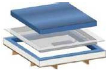
Place the safety liner into the foam frame (the seams should be facing down).
