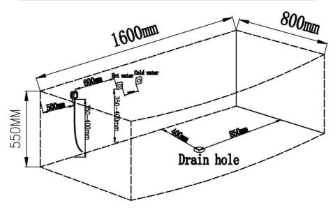
Installation Process Installation Process
