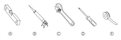
A: Gradient B: Sealant C: Adjustable spanner D: Screwdriver E: PTFE tape
