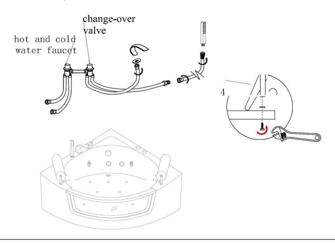
Step 4: as the pics ,First, Take the down-flow pipe inserted into the sewer ,then connect the inlet pipe (take care the hot and cold water ) and Plug the power cord into
