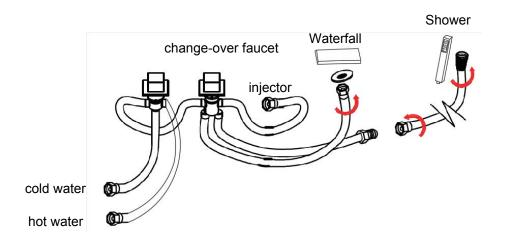
Step 4 : as the pics ,First, Take the down-flow pipe inserted into the sewer ,then connect the inlet pipe (take care the hot and cold water ) and Plug the power cord into
