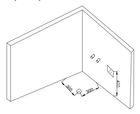
Step 2: Put the bathtub in the corresponding position, leveling with leveling instrument
