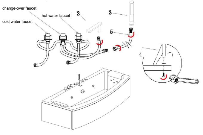
Step 4 : as the pics ,First, Take the down-flow pipe inserted into the sewer ,then connect the inlet pipe (take care the hot and cold water ) and Plug the power cord into
