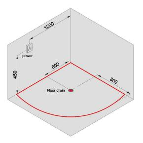
Step 2: Put the bathtub in the corresponding position,
