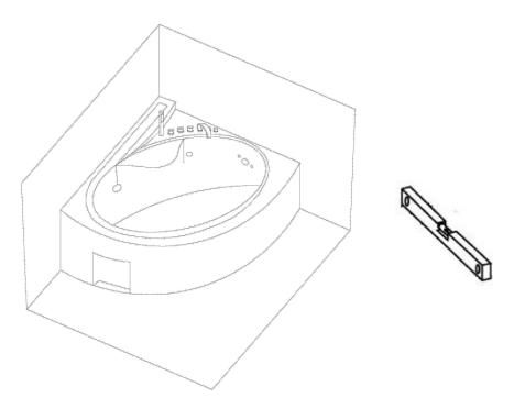
leveling with leveling instrument
