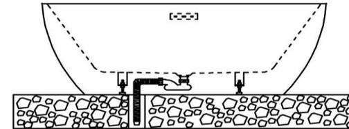
4. After the installation, please do a final test to the bathtub. Please fill the bathtub with water and check if all water flows freely to the waste outlet.
